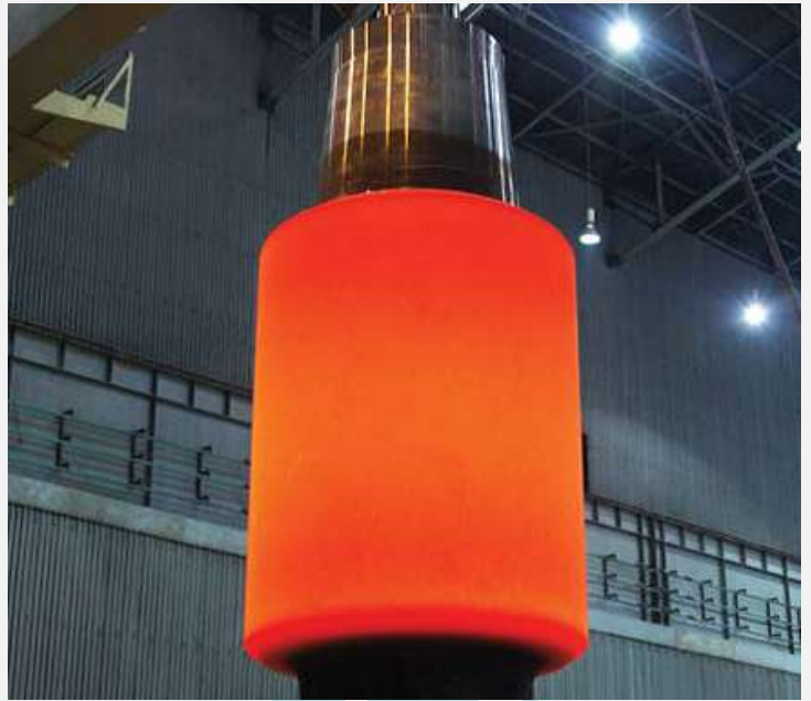
Conventional Heat Treatment of Back-up Roll
